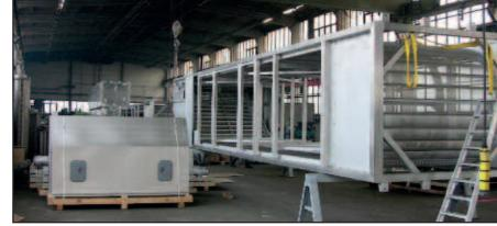
Fish protection technology is a central point in connection with authorisation or operation of plants for water extraction. FSM offers innovative solutions for this area, e.g. travelling band screens/filter belt screens with integrated recirculation and monitoring of fish.
